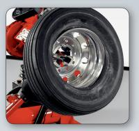
Bead loosening and demounting can be as easy as rolling the tire off of the rim in a single step.
